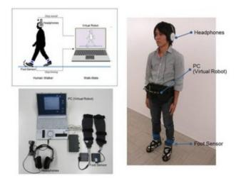
Schematic illustration and components of the WalkMate system. Copyright: Tokyo Institute of Technology
