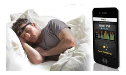
Sleep subjects will use a wireless brain monitor with three sensors incorporated into a headband that will interface with a smartphone.
