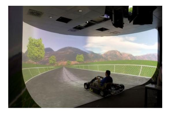
The virtual reality simulation screen extends to 230 degrees horizontally and 125 degrees vertically. The projection fills the whole field of human vision, creating a realistic driving scenario. Credit: Jan Soumann / MPI for Biological Cybernetics
