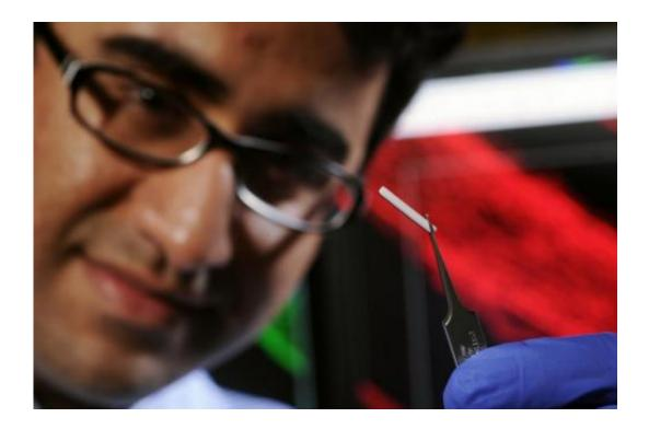
Ph.D. student Nassir Mokarram (left) holds a hollow polymeric nerve guide used to study re-growth of peripheral nerve cells. The nerve guide released interleukin 4 (IL-4) which enhanced the growth of peripheral nerve cells by altering activity of the macrophage cells. Credit: Gary Meek
