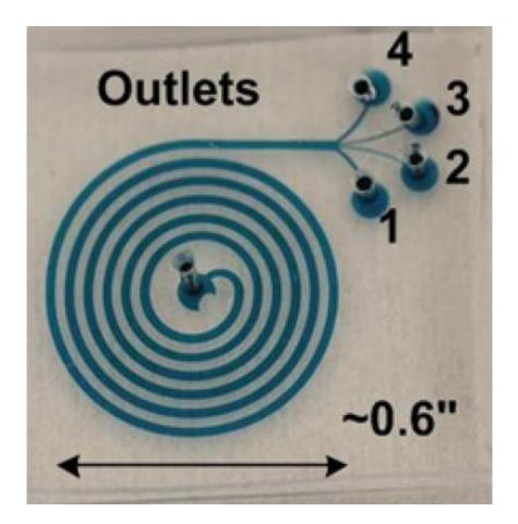
Microfluidic device with spiral microchannels contains four outlet ports which separates blood into different streams. Credit: Nivedita Nivedita, University of Cincinnati
