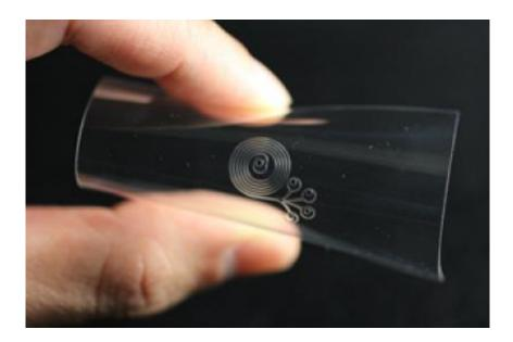
This is another view of microfluidic device with spiral microchannels and four outlet ports which separates blood into different streams. Credit: Nivedita Nivedita, University of Cincinnati
