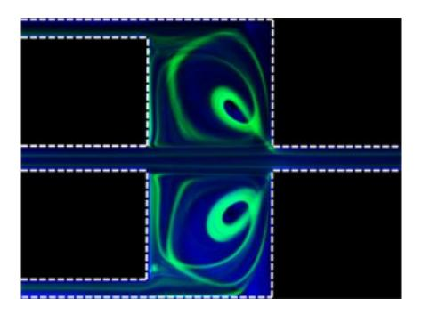
This image shows the size-dependent extraction of particles. The fluorescent image indicates trapping of larger particles while smaller particles pass through. Credit: Xiao Wang, University of Cincinnati
