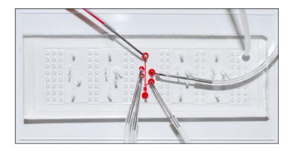
The microfluidic device the research team used to observe the flow-dependent clotting behavior.
