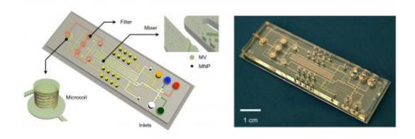
This is a Microfluidic NMR system for the detection of microvesicles (MV) in blood. Labeling with magnetic nanoparticles (MNP) enables detection with a miniature NMR coil. Credit: MGH Center for Systems Biology
