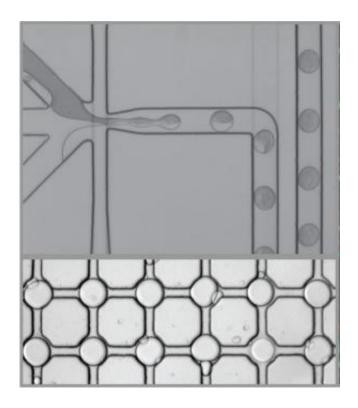
The high sensitivity is achieved by performing the REEAD technology within droplets surrounded by oil. The malaria parasites are distributed in the pico-litre droplet, where they react effectively with the other components of the REEAD technology Credit: Sissel Juul and Birgitta Knudsen
