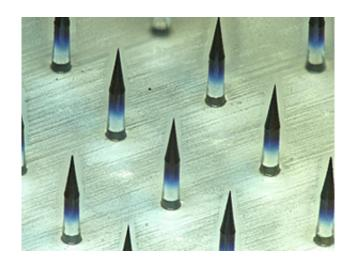
A micro-needle array injected with pigments instead of drugs. Drugs can be injected into the projections (L1000 $\mu$ m x D170 $\mu$ m).
