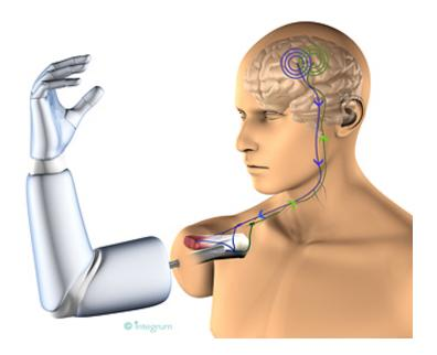
When amputee patients have received their new prosthesis, it will be controlled with their own brain signals. The signals are transferred via the nerves through the arm stump and captured by electrodes. These will then transmit the signals through a titanium implant (OPRA Implant System) to be decoded by the prosthetic arm. The prosthesis is anchored directly to the skeleton by a process known as osseointegration. Credit: Integrum
