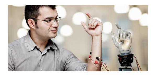
Max Ortiz Catalan demonstrates how the system works with the aid of electrodes, which capture bio-electric signals from the surface of the arm. Amputees will, however, have the electrodes implanted directly on the nerves and muscles inside the body, which will be permanently accessible through the Brånemark osseointegrated implant (OPRA Implant System). Credit: Oscar Mattsson
