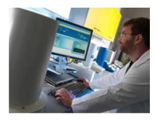
The secondary standard ionisation chambers at NPL that were used in the establishment of traceable 177Lu measurements at hospitals.
