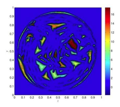
Cross section of a tobacco plug showing heat flow, based on microCT scans and simulations.
