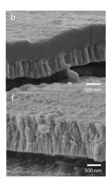
The top scanning electron microscope image (b) shows a cross section of the bioactive hydroxyapatite/YSZ coating without heat treatment. Note how the two
