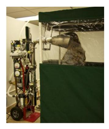
The Gesundheit II machine collects the breath exhaled from flu sufferers. Study volunteers sit for 30 minutes with their heads in the horizontal cone attached to the machine, which sucks in the air around their heads to collect tiny airborne droplets generated deep in the lungs. Researchers can then analyze the aerosols for the presence and quantity of virus. Credit: Donald Milton
