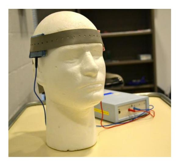
Researchers place the electrodes of this tDCS system so that the current passes through the area of the brain being studied.
