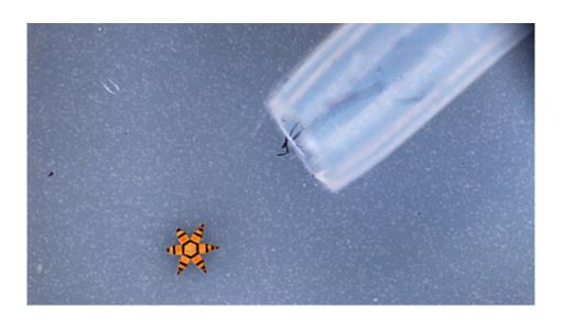
This image depicts an mu-gripper near the opening of an endoscopic catheter. Credit: Evin Gultepe, Gracias Lab, Johns Hopkins University.
