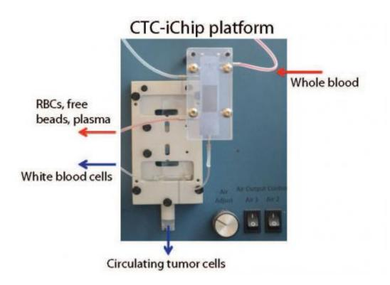
Antigen-independent cell sorting begins by tagging the white cells in a blood sample with magnetic beads. The sample is then passed into the CTC-iChip microfluidic system, which first removes red cells, plasma and free magnetic beads and then sorts out tagged white blood cells, leaving a purified solution of circulating tumor cells. Credit: Emre Ozkumur, Mass. General Hospital Center for Engineering in Medicine
