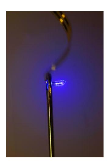
A thin plastic ribbon printed with advanced electronics is threaded through the eye of an ordinary sewing needle. The device, containing LEDs, electrodes and sensors, can be injected into the brain or other organs. Credit: John A Rogers, University of Illinois/Beckman Institute
