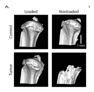
3-D microCT reconstructions of control and tumor-injected tibiae, loaded and nonloaded. Credit: Fischbach lab
