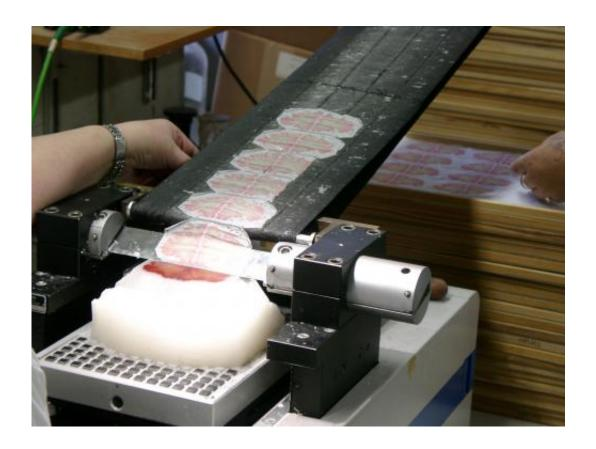
Researchers use a special tool called a microtome to cut sections from a brain preserved in paraffin wax into tiny slivers 20-micromters thick. The researchers cut the brain into over 7,400 such sections. Each highly-folded section was stained to detect cell bodies. Credit: Amunts, Zilles, Evans et al.
