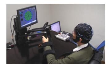
A user operating the brain–computer interface stroke rehabilitation system. Credit: 2013 A\*STAR Institute for Infocomm Research
