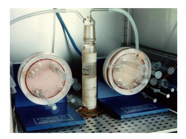
Time-lapse exposure of Bioreactor rotation. The bioreactor is a special incubator that gently spins to circulate cells' growth medium, while preventing turbulence that can harm the cells. (NASA/Dennis Olive)
