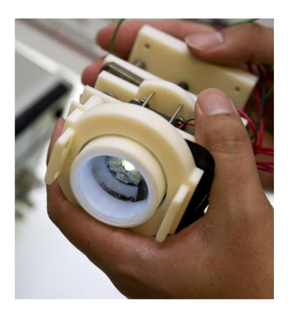
The students' device applies an adhesive film to the breast tissue before it is sliced for examination. The film prevents damage to the samples. Credit: Will
