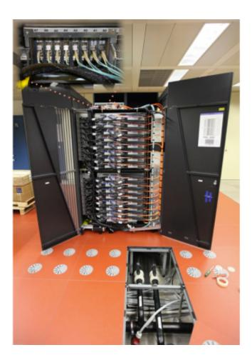
This image shows IBM Blue/Gene Q with a zoom photo of the I/O Subsystem. IBM, EPFL, and ETH are collaborating on a new hybrid memory strategy for supercomputers using both flash and DRAM. When the new memory is installed in the Fall 2013 at the Swiss National Supercomputing Center it will efficiently integrate 128 terabytes of flash memory with 64 terabytes of DRAM memory. Credit: IBM Research
