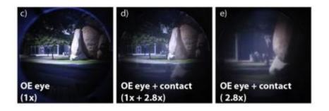
Images captured through the contact lens and mechanical model eye are shown. c) Outdoor image taken with model eye alone. d) Outdoor image taken with model eye and contact lens. This image shows why each of the two magnification states (normal and 2.8x) should be used one at a time: Here,
