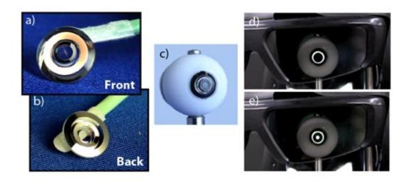
This image shows five views of the switchable telescopic contact lens. a) From front. b) From back. c) On the mechanical model eye. d) With liquid crystal glasses. Here, the glasses block the unmagnified central portion of the lens. e) With liquid crystal glasses. Here, the central portion is not blocked. Credit: *Optics Express*
