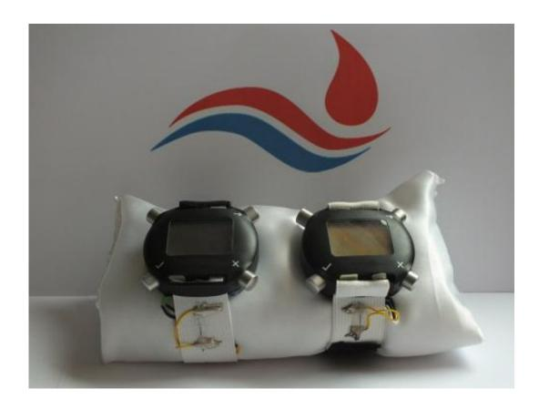
These are the initial prototypes of the "blood pressure watch" with the Empastrap made from piezo-resistive fibres. Credit: Empa
