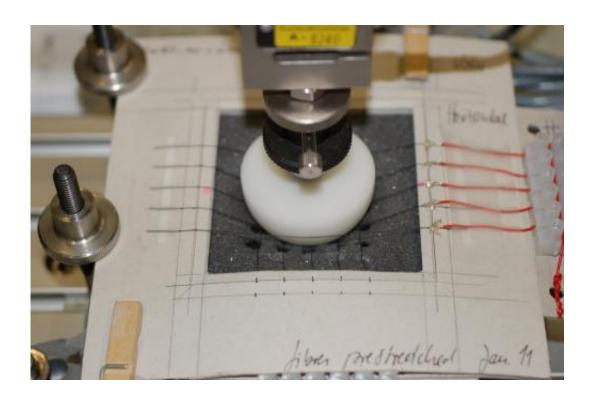
The fibers for measuring contact pressure are produced at Empa. A constant current flows through the individual fibers; if the fibers stretch, their electrical resistance changes. Credit: Empa
