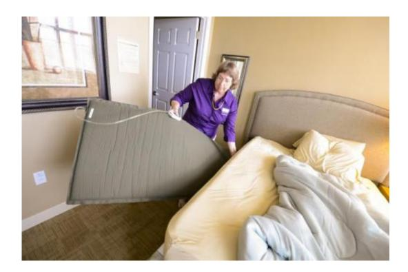
USF College of Nursing's Meredeth Rowe places one of the monitoring device's sensors beneath the mattress. The sensor detects movement and sounds an alarm to alert the caregiver if the person with Alzheimer's disease starts to get out of bed. Credit: © University of South Florida
