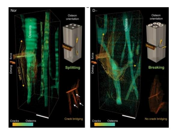
These 3-D reconstructions of crack paths show in the normal bone (left) pronounced crack deflection by splitting along the interfaces of the osteons accompanied by the formation of crack bridges. In vitamin D-deficient sample, the crack takes a tortuous breaking path across the osteons with no crack bridging. Credit: Ritchie and Bale, Berkeley Lab
