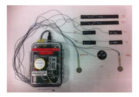
This is the portable device that tracks fluid volume changes. The electrodes, at right, are fastened to a patient's leg and transmit data to the device Credit: Joan Sanders, U of Wash.
