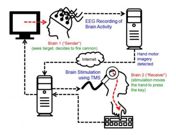
This image shows the cycle of the experiment. Brain signals from the "Sender" are recorded. When the computer detects imagined hand movements, a "fire" command is transmitted over the Internet to the TMS machine, which causes an upward movement of the right hand of the "Receiver." This usually results in the "fire" key being hit. Credit: University of Washington
