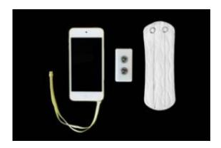
The toilet-training device consists of an iPod, transmitter, and a pad/sensor. Credit: Brandon Vick/University of Rochester
