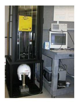
This grandfather-clock-sized machine is so powerful it shakes the floor when it drops its weight onto a helmet.
