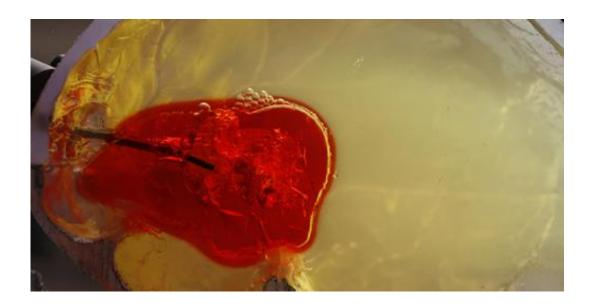
This image shows the test of a steerable needle robotic surgery system on phantom blood clot made from gelatin. Credit: Joe Howell, Vanderbilt
