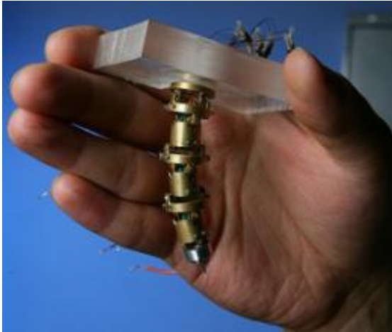
Initial prototype for the minimally invasive neurosurgical intracranial robot. Credit: University of Maryland
