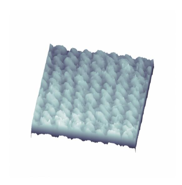
This is a laser microscope image of denim. When we run our fingers along a surface, variations in the surface produce vibrations in the skin which are conveyed as information about texture to the brain. Credit: Bensmaia/University of Chicago
