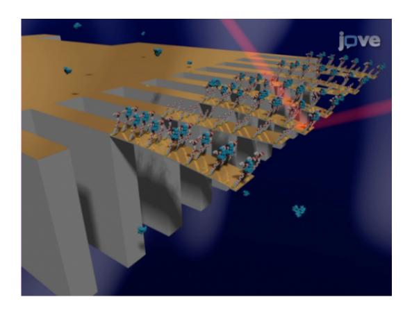
This is a visualization of cantilever sensory array technology. Bacteria are shown in red and white, and antibiotics are shown in blue. The laser deflection illustrates how cantilever bending is measured. Credit: *JoVE*
