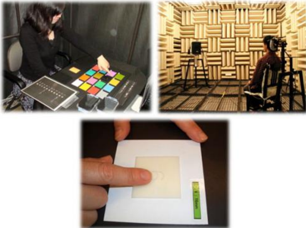
Figure 2 : Examples of sensory characteristic measurements (Upper left) Measurement of vision using standard color samples (Upper right) Measurement of hearing in anechoic chamber (Bottom) Measurement of touch using embossed characters. For example, when measuring the sense of vision, colors that are
