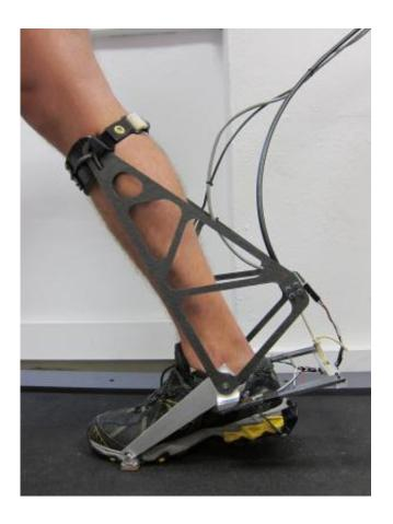
An ankle interface for the assistive ankle robot simulator is being developed at North Carolina State and Carnegie Mellon University. Credit: Steve Collins, Carnegie Mellon University
