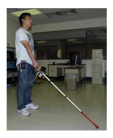
This is a current co-robotic navigation aid prototype used for data collection for preliminary studies. Credit: Cang Ye, Ph.D., University of Arkansas at Little Rock
