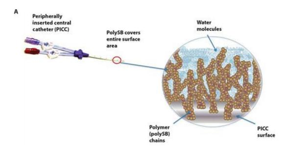
Semprus BioScience's biomaterial, called polySB, sprouts a thicket of polymers (pictured on the right) that attract water molecules, creating an impenetrable barrier against microbes. Credit: SEMPRUS BIOSCIENCES
