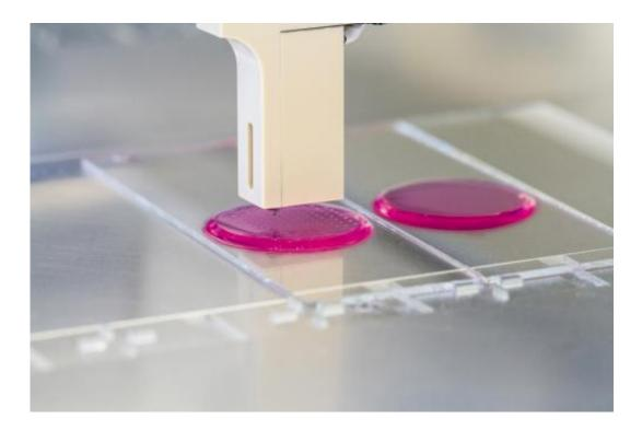
In the lab instead of at the office: researchers using inkjet printers to print cell suspensions onto shimmering pink hydrogel pads, which prevent desiccation. Credit: © Fraunhofer IGB
