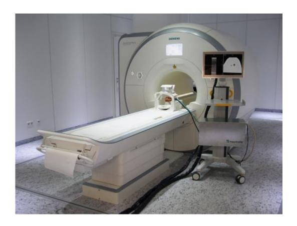
This shows an MR-compatible ultrasound research platform for multimodal imaging and a combination of the advantages of MR imaging and ultrasound imaging for ultrasound-supported movement tracking of internal organs during MRT imaging. Credit: Fraunhofer IBMT
