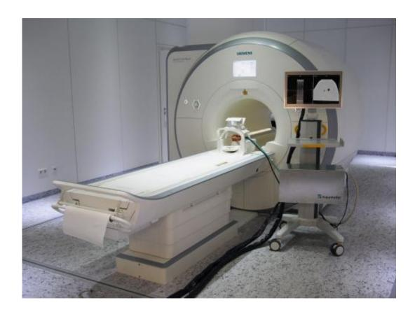
This shows an MR-compatible ultrasound research platform for multimodal imaging and a combination of the advantages of MR imaging and ultrasound imaging for ultrasound-supported movement tracking of internal organs during MRT imaging. Credit: Fraunhofer IBMT
