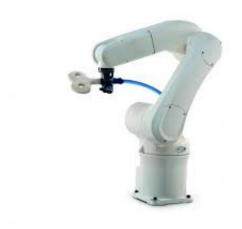
TMS positioning robot. Credit: ant-neuro.com
