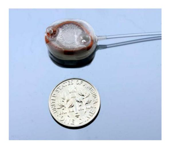
FluidSync implantable infusion micropump sized for use in animals as small as mice. Credit: Ellis Meng, University of Southern California
