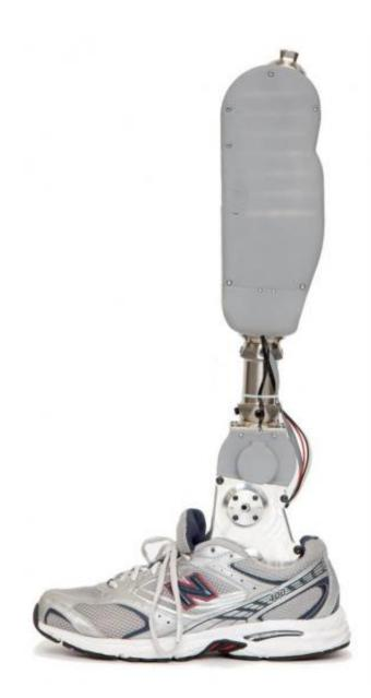
This is a pre-commercial version of the Center for Intelligent Mechatronic's robotic leg, the first lower limb prosthetic with powered knee and ankle joints. Credit: Center for Intelligent Mechatronics, Vanderbilt University
