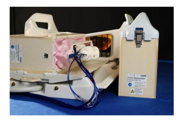
This is the IGAR manipulator and full breast intervention platform mounted on the patient support structure with a biopsy tool attached. Credit: CSii and MDA
