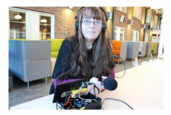
The box in the photo contains the components that will be replaced by electronics in the headset, including the program that communicates with the user during the hearing test. This program will be in the form of an app. The microphone will also be incorporated into the headset. Credit: SINTEF
