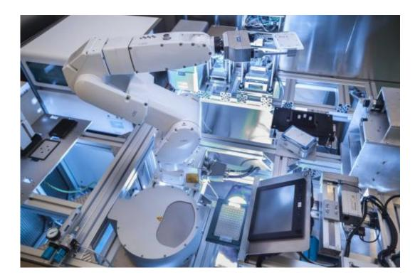
IPA has developed the means to simultaneously measure RNA molecules specifically and precisely from tiny samples of many specimens at once. Fully-automated facility for validation of biomarkers. Credit: Fraunhofer IZI
