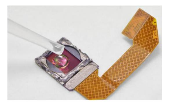
The test sample is placed directly on the exposed surface of the image sensor chip after removal of the optics. The resolution of such mini-microscopes is dependent on the pixel size of the sensor, but sufficient for identification of several pathogenic parasites. Credit: Johan Lundin Lab / Photographer: Heli Vilmi
