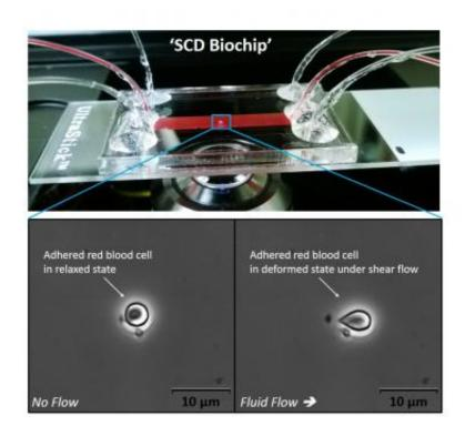
A sticky red blood cell adheres to the surface of a channel in the sickle cell disease biochip. Close-ups show the cell with no flow and with flow. Credit: Umut Gurkan, Case Western Reserve University
