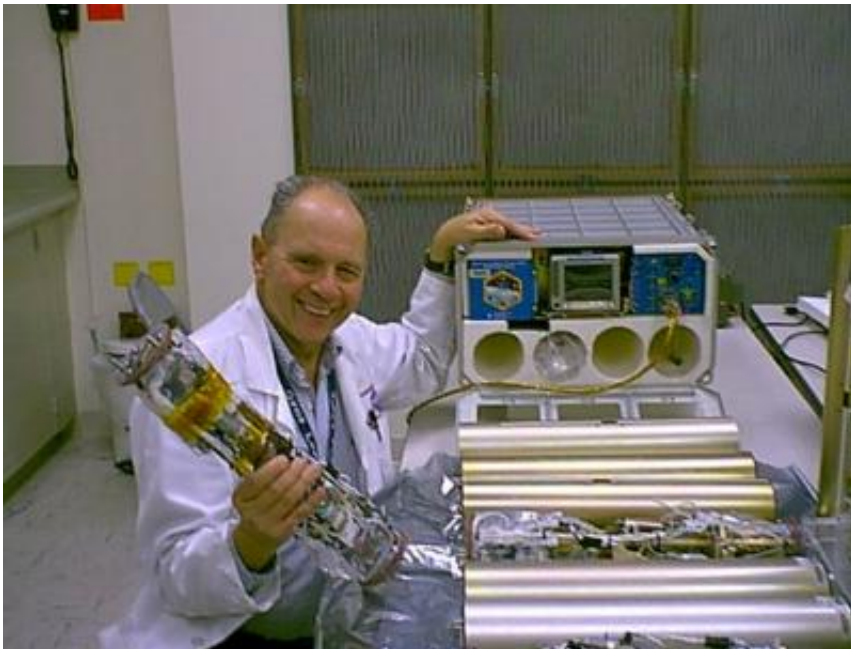
Dr. Dennis Morrison poses with the Microencapsulation Electrostatic Processing System flight hardware that was used on the International Space Station to produce microcapsules for cancer treatment delivery. Credit: NASA
